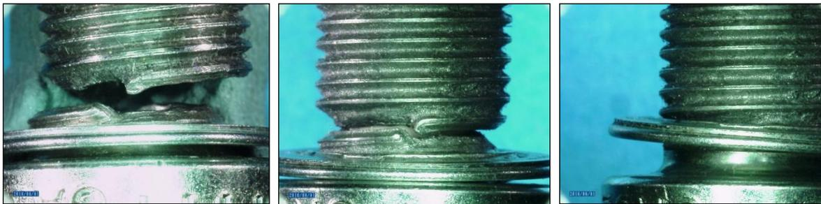
Example of 10mm thread spark plug broken during installation due to the use of anti-seize leading to over-tightening. (Note that plug gasket has been completely compressed, anti-seize can be seen on threads, and the break is in the direction of tightening).
