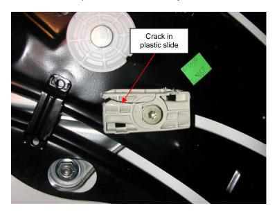
Fig. 21 Failed plastic slide
