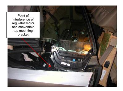
Fig. 19 Window/regulator partially removed
