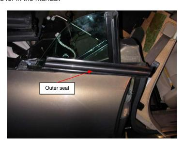
Fig. 15 Window outer seal
