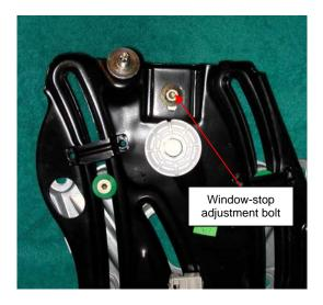
Figs. 22a and 22b View of window stop and adjustment bolt
