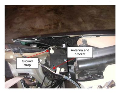
Fig. 16 Alarm antenna, support bracket and ground strap
