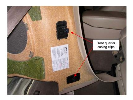
Fig. 8 Clips on front edge of rear quarter casing
