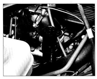
**Diagnostic socket** A diagnostic socket is provided in the ignition system harness. This connection and a connection at the ECU will be used in conjunction with a POD for JDS testing.
