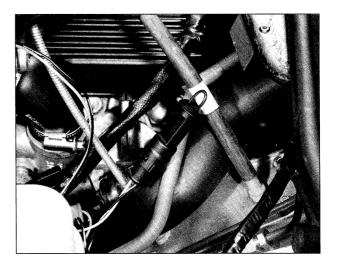
Strategy selection link The ECU memory contains two ignition strategies—one for high octane fuel and one for lower octane fuel. With the link installed, the high octane strategy is selected. With the link removed, the low octane strategy is selected. The strategy selection link should remain installed and the vehicle operated on unleaded premium gasoline.
