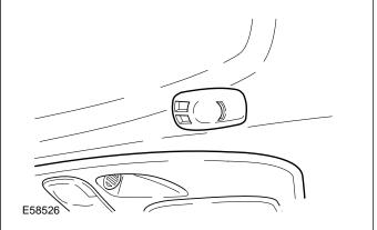
The microphone is located above the driver and is attached to the headliner.
