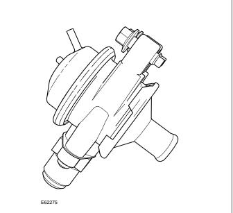
Forced air from the secondary air injection pump is controlled by the secondary air injection control valve. This allows the correct amount of air to be injected directly into the exhaust manifolds. The secondary air injection control valve prevents exhaust gases from blowing back into the secondary air injection pump.
