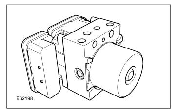
This model year (MY) vehicle sees the introduction of two variants of the hydraulic control unit and anti-lock brake system (ABS) module. The two hydraulic control unit and ABS modules are for non-adaptive cruise control (ACC) and ACC equipped vehicles.
