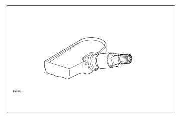
The TPMS system uses 'active' tire low pressure sensors which are mounted on each wheel, inside the tire cavity. The sensor is retained in position by the valve attachment to the wheel structure. The sensors transmit RF signals at either 315 MHz or 433 MHz dependent on market requirements.
