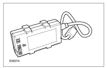
The Bluetooth upgrade module has one electrical connector and communicates with the PSE module by it's own proprietary communications bus.
