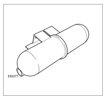
A secondary air injection vacuum reservoir is located on the right-hand side of the engine bay. The secondary air injection vacuum reservoir is included in the vacuum supply line between the intake manifold and the secondary air injection vacuum solenoid valve.
