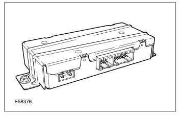
The voice activated control module is fixed to a bracket which also supports the PSE and the navigation control module.
