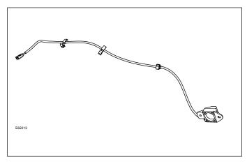
The TPMS external antenna is located at the rear of the vehicle and is mounted between the spare wheel well and rear subframe.
