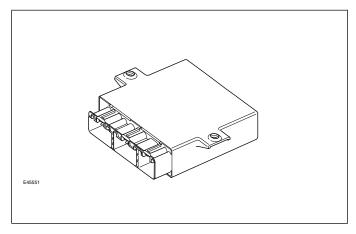
The TPMS module is located in the left-hand side of the spare wheel well. The TPMS module is fixed in position to a shared mounting bracket using a retaining nut. The connectors of the TPMS module point downwards and the external antenna connector points upwards.
