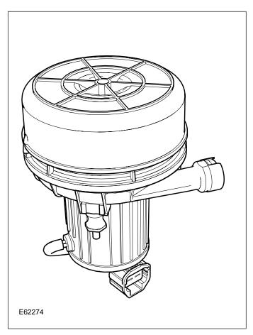
The secondary air injection pump is located behind the left-hand side of the front bumper cover. The pump is fitted on rubber mountings to help suppress noise generated by secondary air injection pump operation. The secondary air injection pump is powered from the battery by a dedicated relay and supplies approximately 10-15 kg/hr (22-33 lb/hr) of air when the vehicle is at idle on initial start up from 20°C (68°F).
