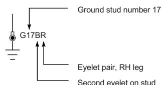
On figures where LHD and RHD circuits are combined and the ground designation differs from LHD to RHD, the RHD ground code is shown in parentheses. If the ground designation is the same for LHD and RHD, only one ground code is used, with no parentheses.
