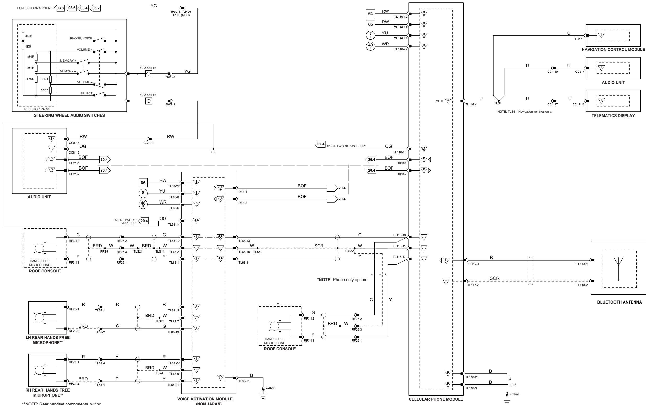
\*\*NOTE: Rear handset components, wiring and circuitry – Multi-zone Voice vehicles only.
