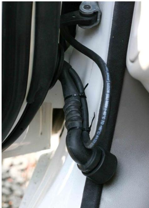
**Step 23:** Cutoff the tie wrap tails. Take the loose end of the cable and push the remaining cable through the adjacent open cavity of the fender. Reinsert the grommet in the door, and rotate the boot back to its original position. Re-insert the round connector into the body with a clockwise turn until it stops. The final product should look like the photo below, with the new cable tie wrapped behind the boot and barely visible:
