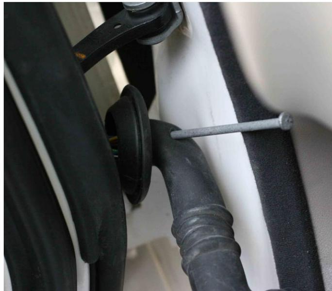
**Step 21:** Spray a small amount of silicone lubricant on one end of the 15 foot rubber line cord. Force it through the pierced hole. from the outside. Pull about 4-5 feet of cable through and thread it through the exact same path as the other wiring harnesses in the door. Tie wrap it to the other harnesses along the way.
