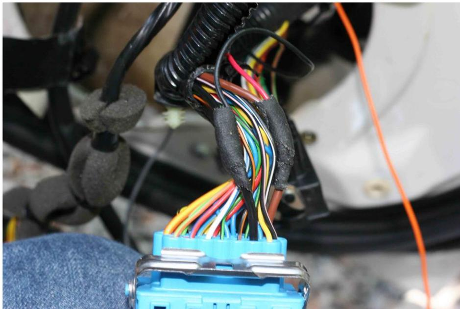
**Step 12:** Continuing with DD10, the blue connector, solder tap the yellow wire (DD10, terminal 5) to the orange wire from the relay/timer wire assembly. Double check this is the SOLID yellow wire on terminal 5, and not a yellow wire with a colored stripe. See below.
