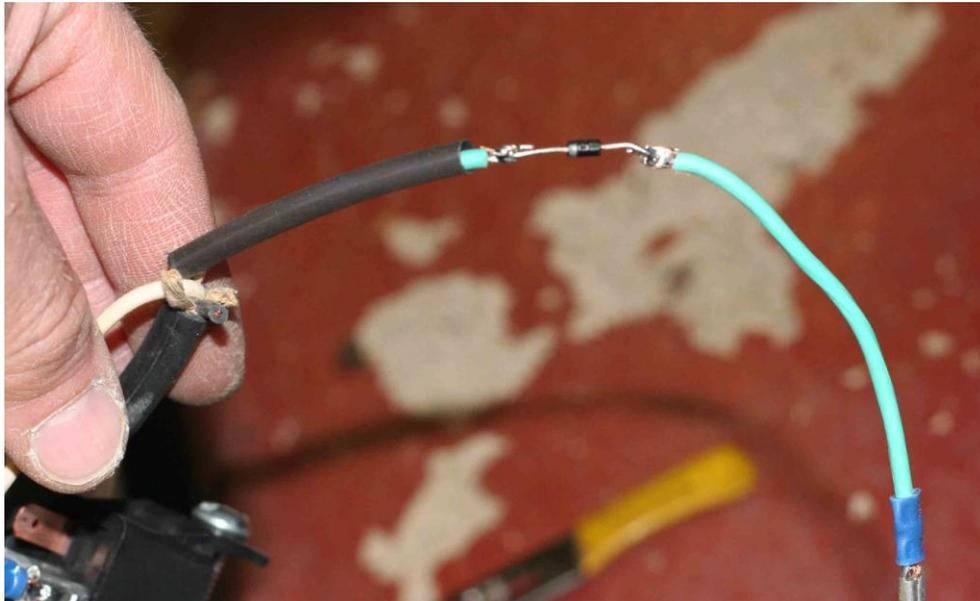
**Step 36:** Fold the diode back over the black line code cable jacket and tape it in place with electrical tape. This will provide protection and strain relief for the diode.
