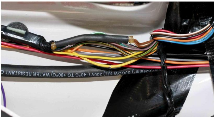
**Step 16:** Pull the violet wire from the relay/timer wire assembly back from the speaker area to the central area of the harness discussed in step 14 above. Solder the CATHODE (white striped side) of a 1N4001 diode to the LEFT side of the cut yellow wire AND to the violet wire. Slide on heat shrink tubing. Solder the ANODE of the diode the RIGHT side of the yellow wire. This is illustrated below photos:
