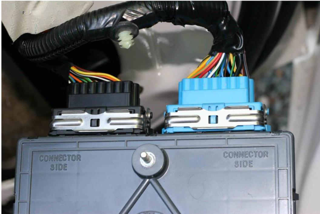
**Step 7:** Remove the black and blue connectors from the Driver Door Module. To remove a connector, depress the square button while lifting the metal tab end nearest the module upwards. The connectors will self-extract during this process.
