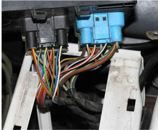
**Step 33:** Route the line cord cable from the wheel well to the fusebox and up through the opening underneath it. Strip the outer rubber insulation about 4 inches back. Solder tap the green wire from the rubber line cord to the green/red wire on the black connector LF6, terminal 9. Solder tap the white wire from the rubber line cord to the red/white wire on the blue connector LF8, terminal 8. The black wire in the rubber line cord can be cut back to the outer jacket, it is not used.
