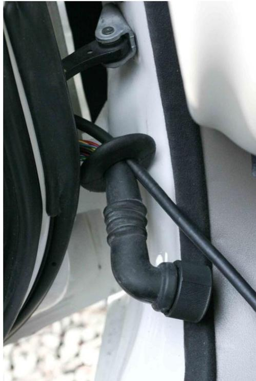
**Step 22:** Neatly dress the cable to the boot with two black tie wraps as show below:
