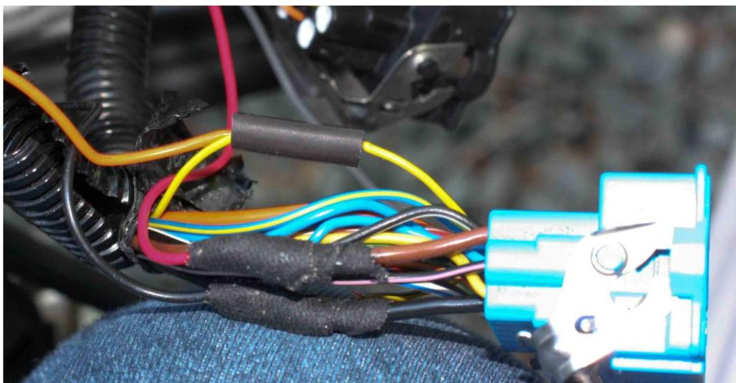
**Step 13:** Moving on to the black connector, DD11, locate terminal 4, the green wire with a brown stripe. Solder tap this wire to the grey wire from the relay/timer harness. See below.
