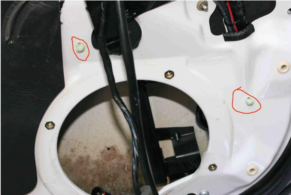
**Step 5:** Remove the three 7mm bolts retaining the Driver Door Module behind the sheet metal of the inner door (note: your wiring will look different...some of these photos were taken after the new wiring was added).
