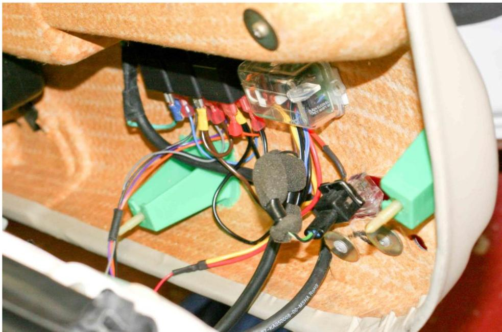
**Step 40:** Reinstall the puddle lamp connector. Reassemble the door panel trim and hardware on the door per the video instructions from Rev. Sam.
