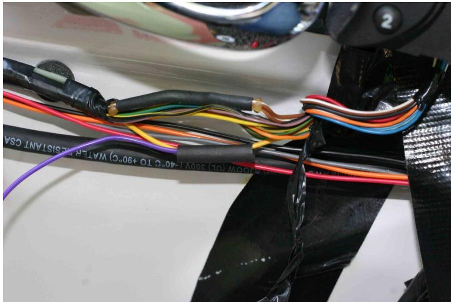
Shrink the tubing with a heat gun and re-tape the harness with vinyl electrical tape.
