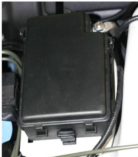
**Step 32:** Tilt up the fusebox, exposing the blue and black connectors on the underside.
