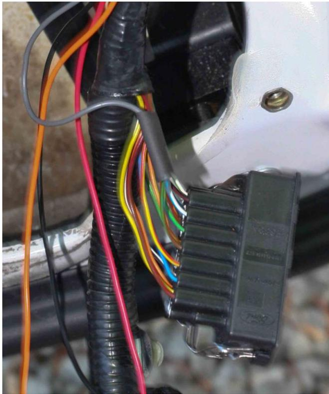
**Step 14:** Re-tape both of the Driver Door Module connector harnesses with vinyl electrical tape up to near the connector bodies.
