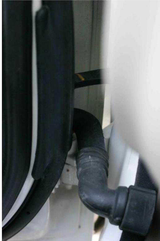
**Step 20:** Carefully pierce the rubber boot precisely as shown in the photo below with awl or sharp nail. Be very careful not to damage wires in the boot.
