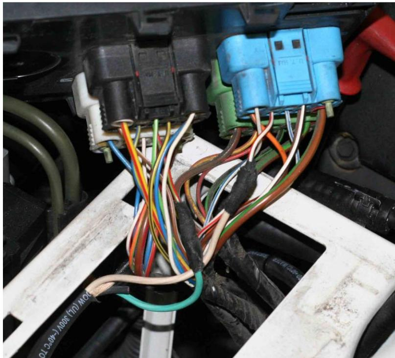
**Step 34:** Wrap each harness in vinyl electrical tape, taking care to cover the solder taps. Reinstall the fuse box, sliding it forward in its mount and depressing the latch. Reinstall the ground cable, and rubber cover. Shut the hood.
