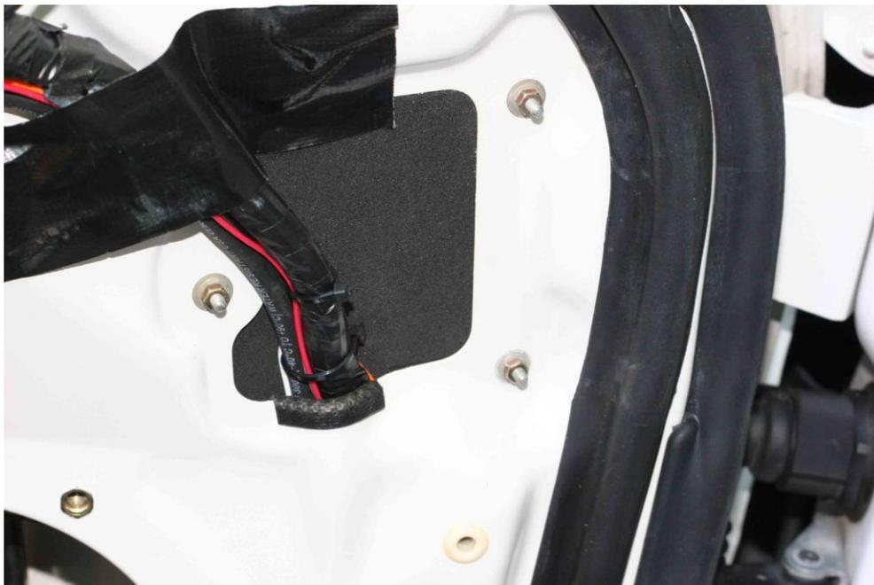
**Step 6:** Carefully extract the driver door module from the inside of the door cavity with the attached cables through the speaker opening. Make sure you do not lose the foam gasket inside the door.
