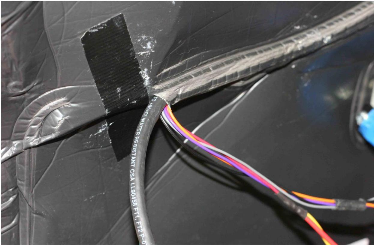
**Step 18:** Apply double faced carpet tape in sections to the back of the vapor barrier in areas where it was previously peeled off. Remove the tape backing and restore the vapor barrier to its original position adhered to the inner door.
