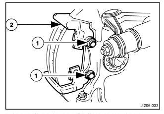
7. Remove the caliper carrier from the vertical link.
