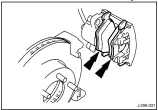
6. Remove the brake pads from the caliper.
