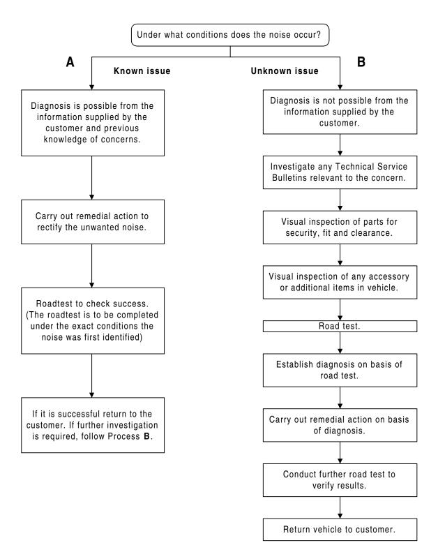
**Note:** If the road test does not provide cause, fax the Squeaks and Rattles Diagnostic check sheet to Technical Hotline and then contact for further assistance.
