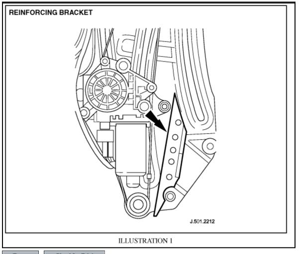
Note: If only one side rear <u>quarter window regulator</u> has failed, inspect the opposite regulator to see if it is equipped with a reinforcing bracket (Arrowed area in Illustration 1.) If not replace both regulators.
