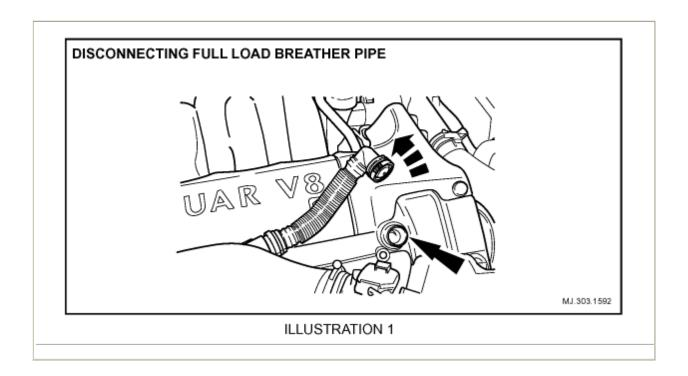
4. Disconnect the full load breather line on the right camshaft cover, (Illustration 1).
