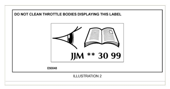
\*Caution: If the <a href="https://example.com/the-body">throttle body</a> displays the label shown in Illustration 2, do not clean the throttle body bore and butterfly valve as damage to the vehicle can result.\*
