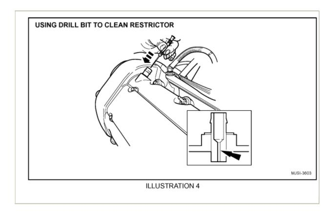
7. Insert a 3/32" (2.5 mm) diameter drill bit in a hand-held pin chuck such as Snap-on Tools(R) Part No. YA 806 (Illustration 4). Verify that the drill bit does not exceed 3/32" (2.5 mm) diameter.
