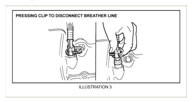
6. Depress the retaining clip (Illustration 3) of the connector of the part-load breather line, allowing the line connector to be disconnected from the breather stub on the left camshaft cover.
