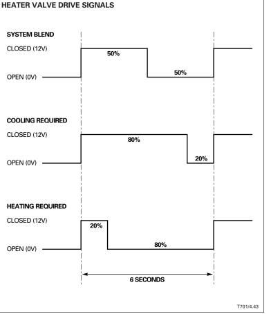
The A/CCM drives the valve with a 12 volt, six second duty cycle signal. The A/CCM increases or decreases the length of the 12 volt signal within the duty cycle to achieve the required heater matrix temperature. If the drive circuit fails (open circuit), the valve defaults to the open position to allow full engine coolant flow to the heater matrix.
