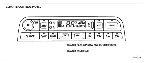
The heated rear window and door mirrors are activated by pressing the "R" button on the climate control panel. The heated windshield can be activated manually by pressing the panel "F" button.
