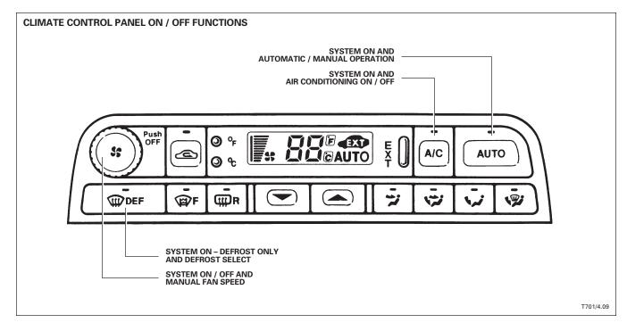
The climate control panel is switched ON by pressing one of the following panel controls:
