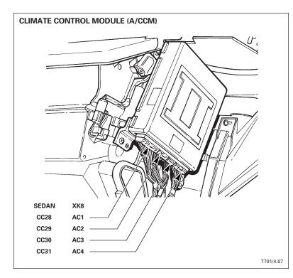
The A/CCM has two microprocessors: one 8-bit and one 4-bit. The 8-bit microprocessor controls the overall system strategy and stores input / output information. The 4-bit microprocessor "conditions" the system signals and processes information.
